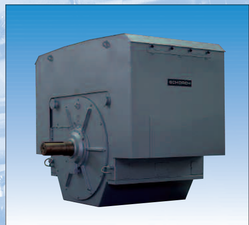
Internally ventilated shredder drive, motor 1,500 kW, 6 kV, 10-pole, with top-mounted weather protection cover, IP24W
