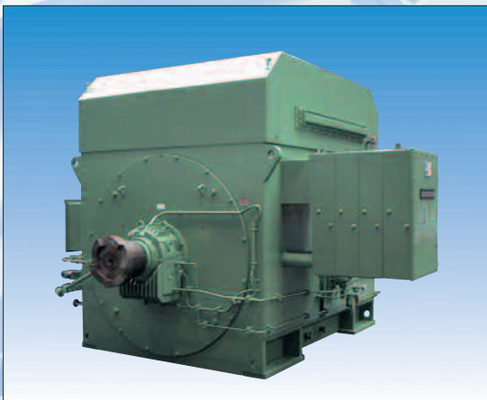
Extruder drive, motor 9,300 kW, 11 kV, 6-pole, IP55, with top-mounted water/air heat exchanger
